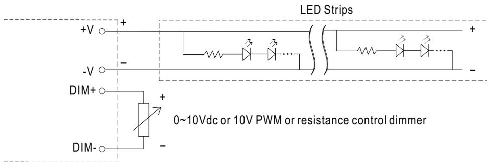
※DO NOT connect "DIM- to -V"
